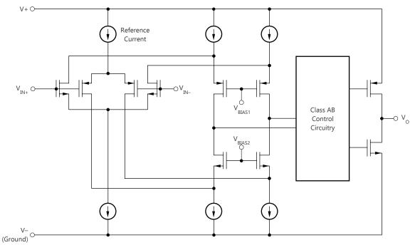
Figure 1-1. Functional Block Diagram
