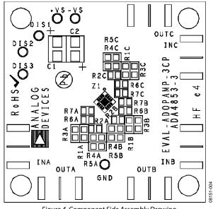
Figure 4. Component Side Assembly Drawing
