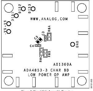
Figure 5. Circuit Side Assembly Drawing
