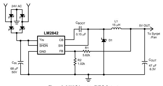
Figure 3. 24VAC Input to 5VDC Output
