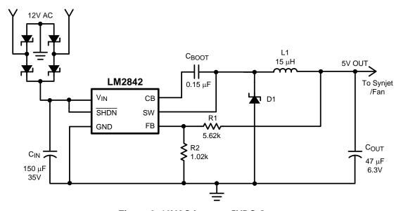
Figure 2. 12VAC Input to 5VDC Output
