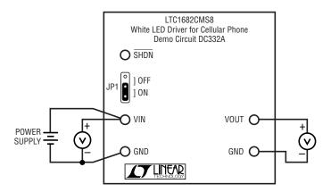
Figure 1. DC332A Test and Measurement Setup
