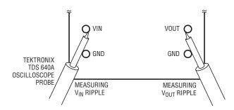
Figure 2. Proper Noise Measurement Technique
