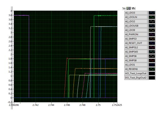
Figure 3. ON Request Using PWRON
