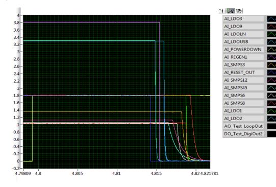
Figure 9. OFF Request Using POWERDOWN
