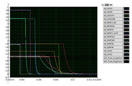
Figure 11. OFF Request Using RESET\_IN
