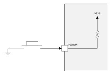
Figure 2. Typical PWRON Configuration
