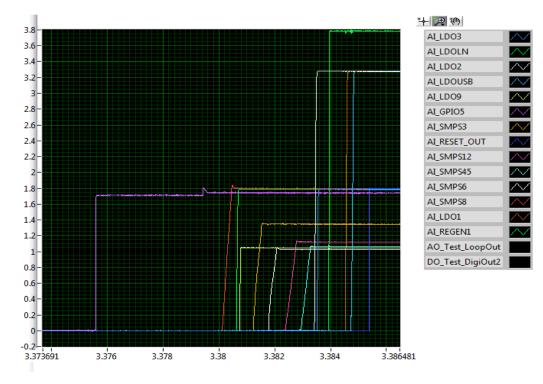
Figure 5. ON Request Using GPIO\_5 Interrupt
