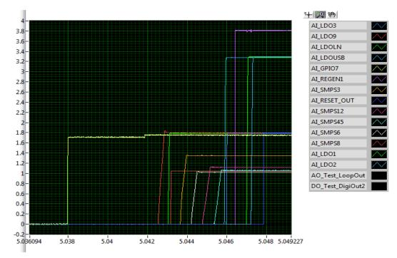
Figure 7. ON Request Using POWERHOLD
