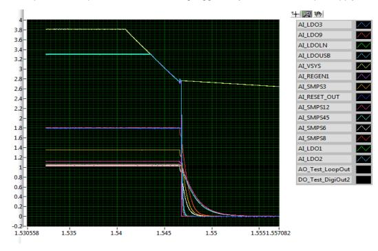
Figure 12. OFF Request by Removal of Supply Voltage (VSYS\_LO)
