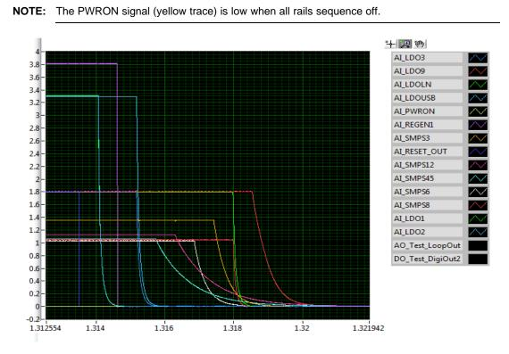
Figure 8. OFF Request Using Long Key Press (PWRON)
