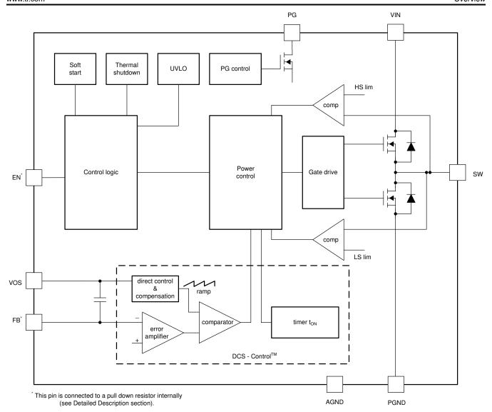
Figure 1-2. TPS62160-Q1 Functional Block Diagram
