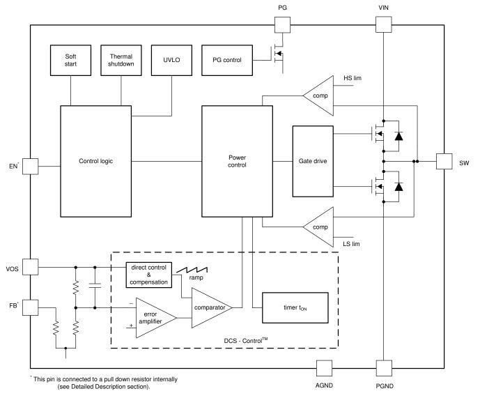
Figure 1-1. TPS62162-Q1 Functional Block Diagram
