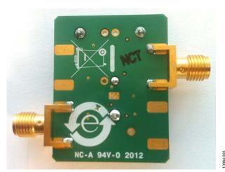
Figure 2. ADA4432-1BCP-EBZ Evaluation Board, Secondary Side
