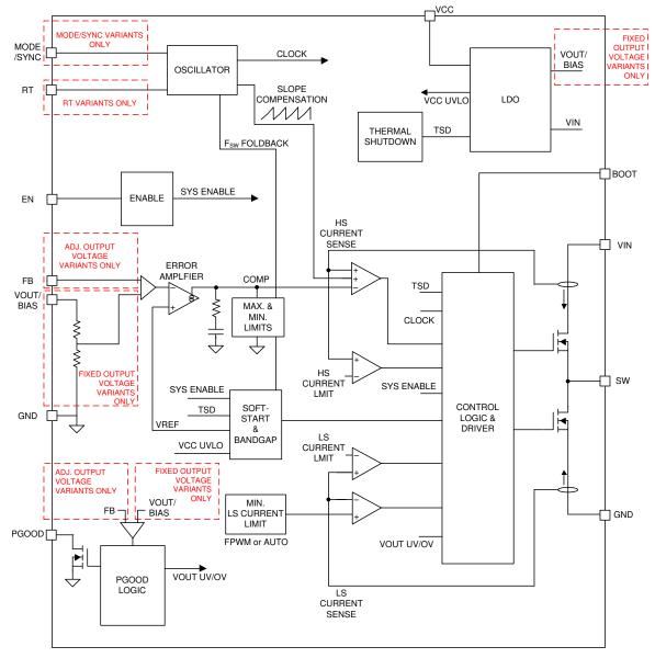
Figure 1-1. Functional Block Diagram
