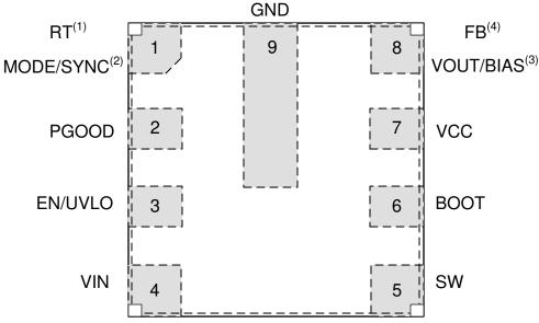
1. See the datasheet for more details. Pin 1 trimmed and factory-set for externally adjustable switching frequency RT variants only.
