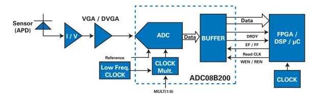
Figure 2. Ranging circuit using the ADC08B200
