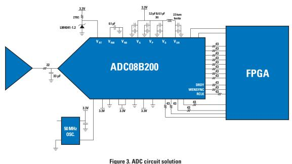
Figure 3. ADC circuit solution
