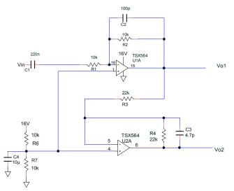
The following picture shows a scope of the input signal amplitude, which has been multiplied by two thanks to the architecture presented in Figure 2. Schematic to drive a resolver. An error of 1.6% can be observed on Vo2-Vo1 signal compared to the theoretical value, mainly due to the matching of the resistance (resistance tolerance1%) see Eq. (13).
