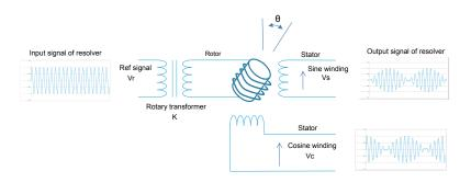
Figure 1. Resolver principle
