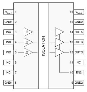
Figure 4-1. Pin Diagram (16-QSOP and 16-DW) Package
