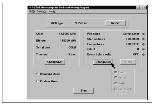
Figure 4.8 Main Window: Write and Erase Setting
