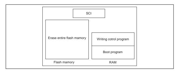
The writing program will acquire an application program from the Serial Communication Interface (SCI), etc. and load it into the flash memory.
