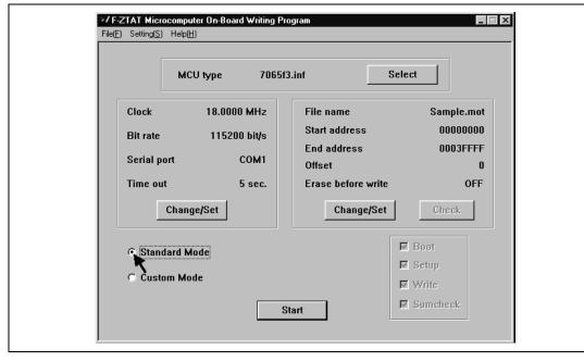
Figure 4.3 Main Window: Selecting the Standard Mode
