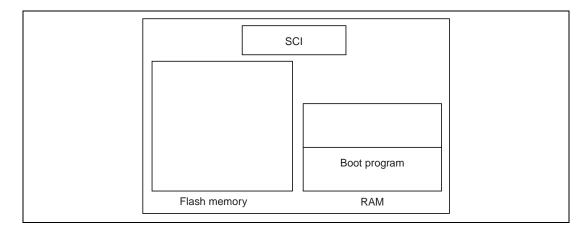
The boot program will acquire the writing program through the Serial Communication Interface (SCI) and load it into RAM.
