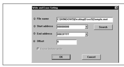
Figure 4.9 [Write and Erase Setting] Dialog Box
