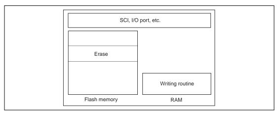
The writing routine will acquire rewriting data from the SCI, I/O port, etc. and writes them to the flash memory. The writing routine can acquire the writing data from arbitrary peripheral functions according to the user system's function.
