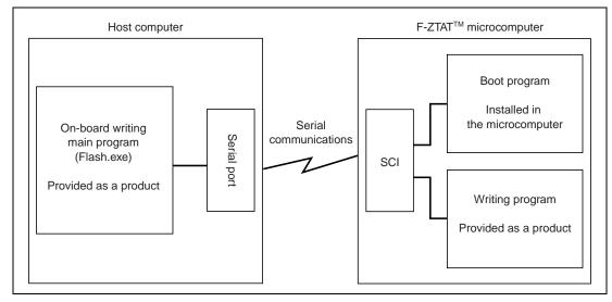
Figure 1.1 Model of Operation of an On-Board Writing Program
