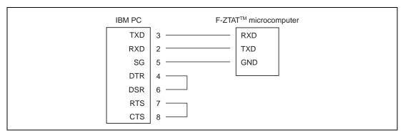
Figure 3.1 Connecting IBM PC Serial Port to SCI (Model)
