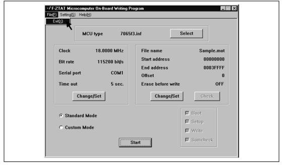
Figure 4.2 Main Window: Ending the On-Board Writing Program
