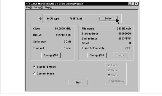
Figure 4.4 Main Window: Selecting the Microcomputer
