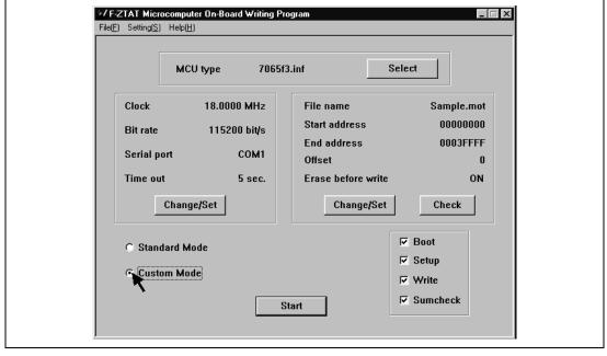
Figure 5.1 Main Window: Selecting Custom Mode
