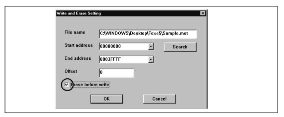
Figure 5.3 [Write and Erase Settings] Dialog Box: Selecting Erase before Write
