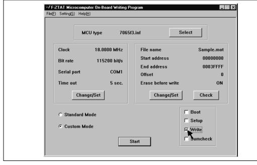
Figure 5.2 Main Window: Selecting Boot/Set up/Write
