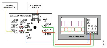
Figure 2. ADN4690E/ADN4691E/ADN4694E/ADN4696E Driver Evaluation with EVAL-ADN469xEHDEBZ
