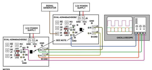
NOTES 1. REPLACE  $50\Omega$  resistors with  $100\Omega$  when evaluating two boards connected together.
