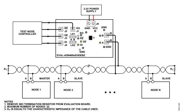
Figure 5. EVAL-ADN469xEHDEBZ Application Evaluation Connected to Bus and Control Board
