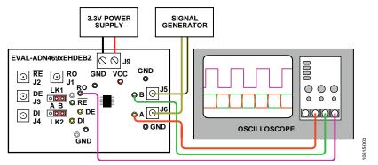
Figure 3. ADN4690E/ADN4691E/ ADN4694E/ADN4696E Receiver Evaluation with EVAL-ADN469xEHDEBZ
