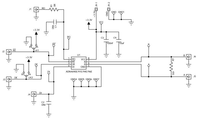
Figure 6. EVAL-ADN469xEHDEBZ Schematic
