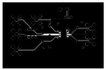
Figure 8. EVAL-ADN469xEHDEBZ Component Side
