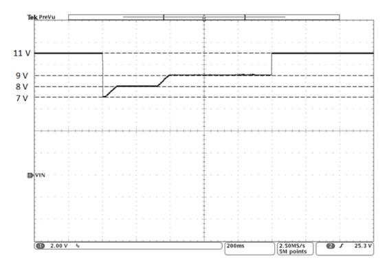
Figure 1. Example of Warm Crank Test Profile
