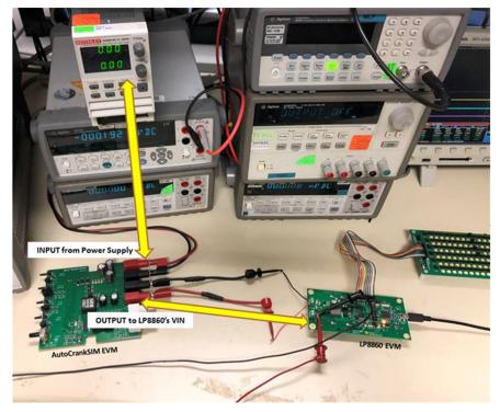
Figure 4. Cold Crank Test Connection
