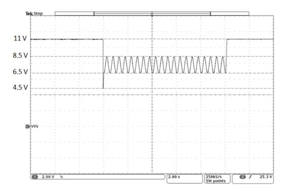
Figure 2. Example of Cold Crank Test Profile
