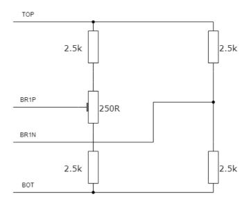
Figure 4: Schematic of the Board Sensor Circuit [4]
