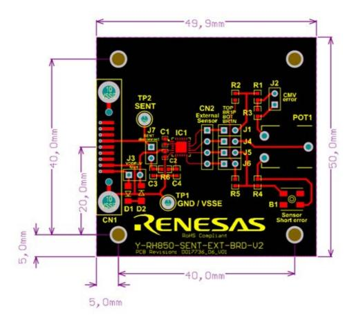
Figure 5: RH850 SENT Application Board dimensions
