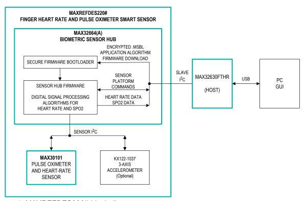
Figure 1. MAXREFDES220# block diagram.
