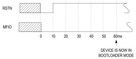
Figure 8. Entering bootloader mode using the RSTN pin and the MFIO GPIO pin.
