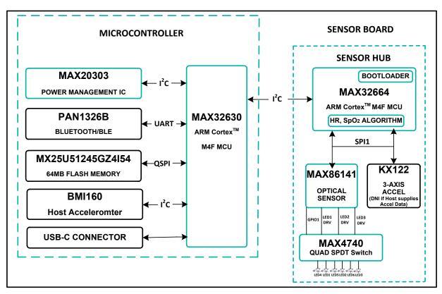
Figure 3. MAXREFDES103# block diagram.
