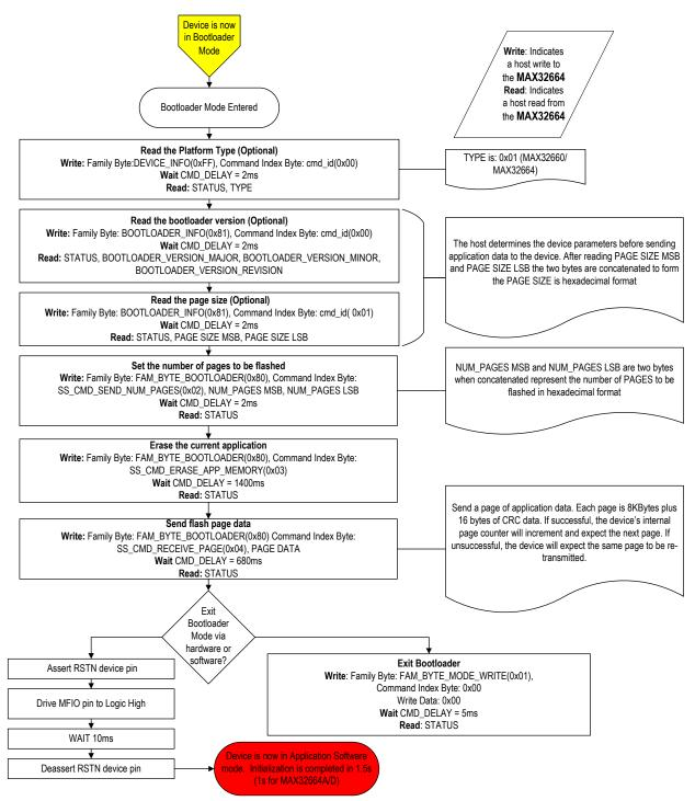
Figure 18. MAX32664 in-application programming flowchart.
