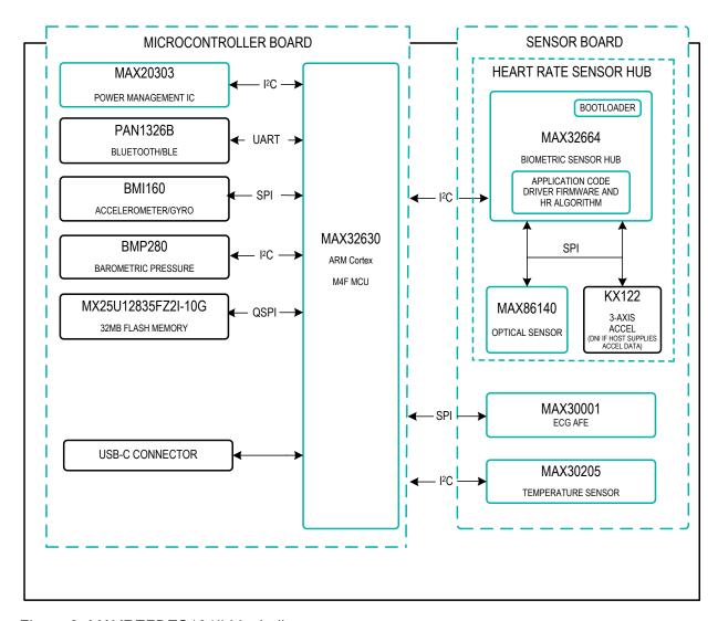
Figure 2. MAXREFDES101# block diagram.
