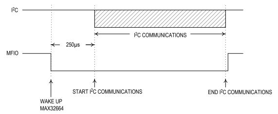
Figure 7. Host sets MFIO low to wake up the low-powered versions of the MAX32664.
