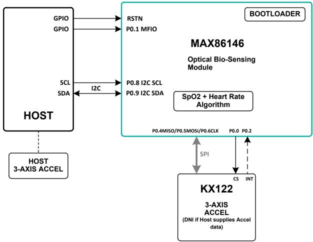
Figure 5. Block diagram for Host, MAXM86146 (Sensor Hub with Integrated AFE and Photodiodes).
