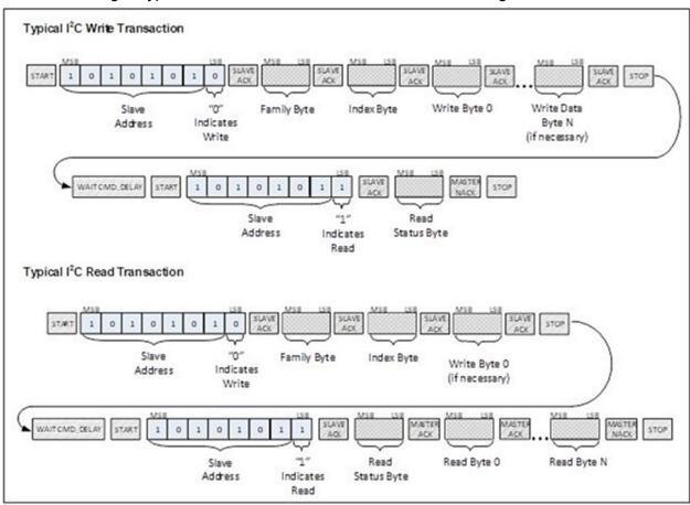
Figure 10. I<sup>2</sup>C Write/Read data transfer from host microcontroller.
