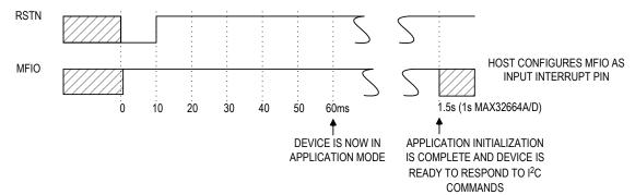
Figure 9. Entering application mode using the RSTN pin and MFIO pin.
