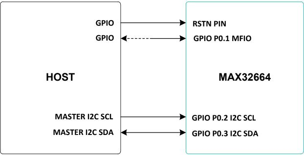
Figure 6. Pin connections between the host and the MAX32664.
