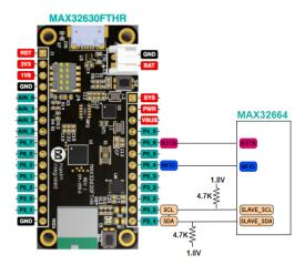
Figure 11. Using the MAX32630FTHR to flash the application .msbl to the MAX32664.
