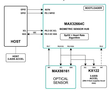
Figure 4. Block diagram for Host, MAX32664C Sensor Hub, and MAXM86161.
