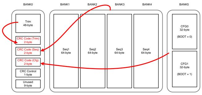
Figure 6. OTP Register Map Diagram
