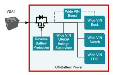
Figure 1. Direct-off battery voltage supervision
