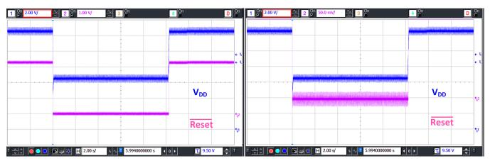
Figure 4. DaimlerChrysler Engine-Cranking Test Pulse, DC-10615
