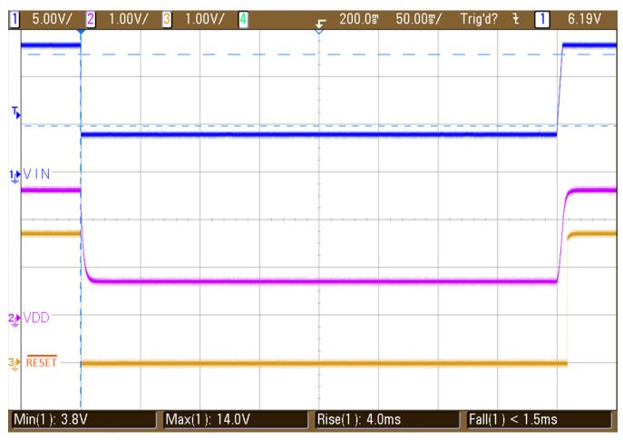
Figure 7. 13.5V<sub>IN</sub> to 4.2V<sub>IN</sub> Transient (Cold-Crank)
