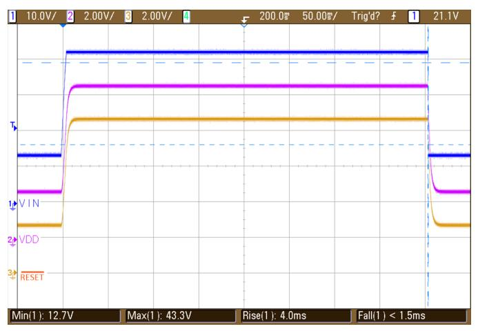
Figure 8. 13.5V<sub>IN</sub> to 42V<sub>IN</sub> Transient (Load-Dump)
