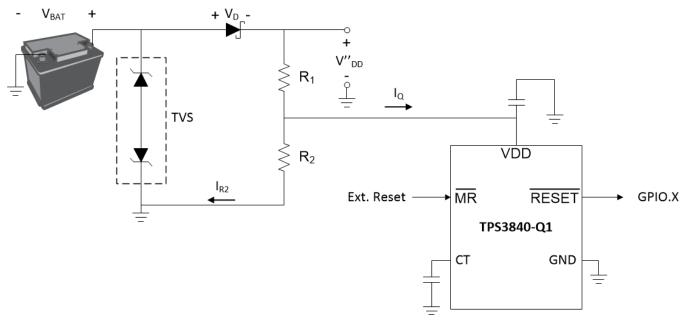
Figure 2. TPS3840-Q1 Schematic
