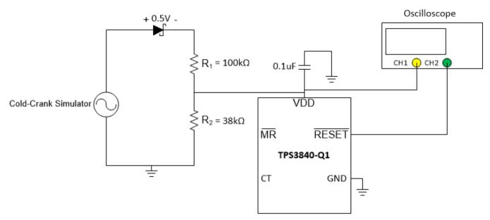
Figure 3. Cold-Crank Test Setup
