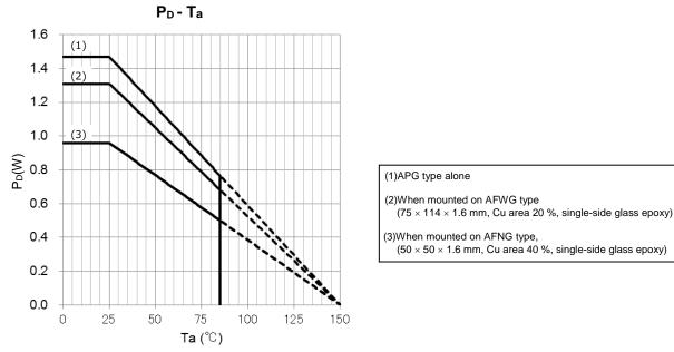
$(50 \times 50 \times 1.6 \text{ mm}, \text{Cu} \text{ area } 40 \%, \text{ single-side glass epoxy})$
