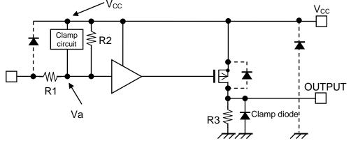
\*Constant number of internal resistance: R1=320.5 k $\Omega$  (typ.), R2=300 k $\Omega$  (typ.)
