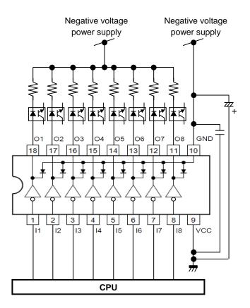
For voltage stabilization and noise rejection, please connect a stacked ceramic capacitor (0.01  $\mu$ F to 1  $\mu$ F) or an electrolytic capacitor (10  $\mu$ F to 100  $\mu$ F) to V<sub>CC</sub> line. The capacitor is recommended to be connected as close to the IC as possible.
