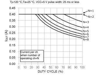
I<sub>OUT</sub> - DUTY CYCLE Mounted on the board of TBD62786AFNG Tj=120 °C,Ta=25 °C, VCC=5 V pulse width: 25 ms or less
