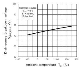
Fig. 8.11 V<sub>(BR)DSS</sub> - T<sub>a</sub>
