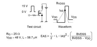
Fig. 8.16 Test Circuit/Waveform
