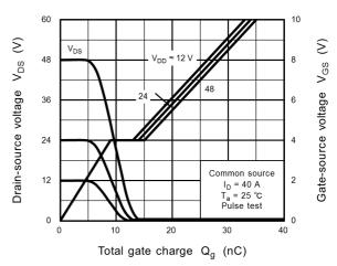
Fig. 8.14 Dynamic Input/Output Characteristics
