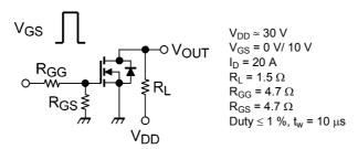
Fig. 6.2.1 Switching Time Test Circuit
