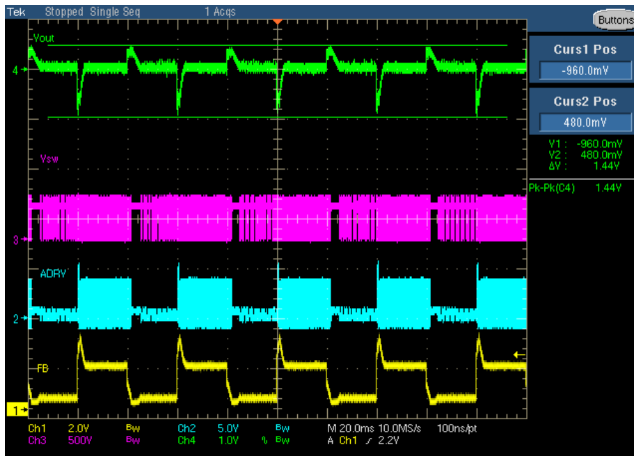
Figure 48. 230 Vac 12 Vout Transient
