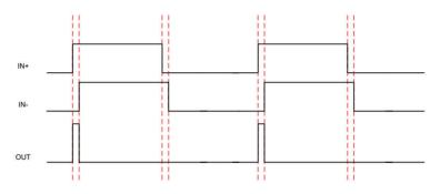
Figure 6. Nano Second Pulse Timing Diagram with Delayed Signal
