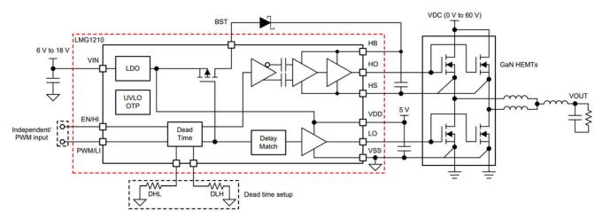
Figure 7. Block Diagram of the Synchronous Buck Converter
