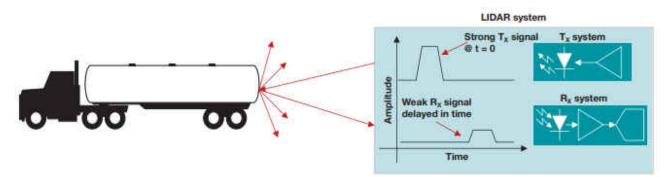
Figure 1. LIDAR Transmission and Receiver Functionality
