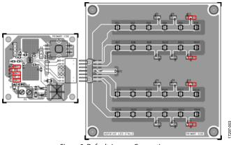
Figure 3. Default Jumper Connections
