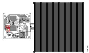
Figure 4. ADP8140EB-EVALZ and ADP8140 LED-EVALZ Connection
