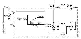
Figure 11. ADP8140 LED-EVALZ Board Current Scaling Using the VT Pin
