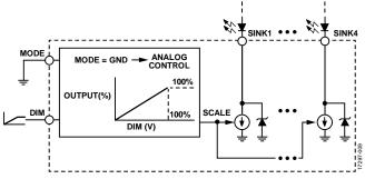
Figure 9. Reduced LED Current Using DC Voltage at DIM Pin
