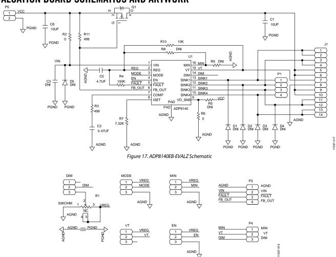
Figure 18. ADP8140EB-EVALZ Schematic Connectors and Peripherals
