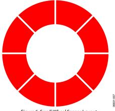
Figure 6. Scroll Wheel Sensor Layout
