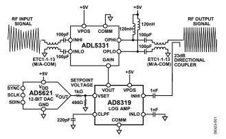
Figure 1. ADL5331 Operating in an Automatic Gain Control Loop in Combination with the AD8319 and AD5621 (Simplified Schematic)
