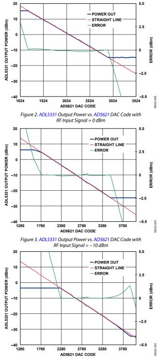
Figure 4. ADL5331 Output Power vs. AD5621 DAC Code with RF Input Signal = -20 dBm
