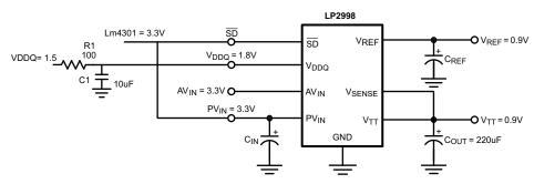
Figure 6. Inrush Current Controlled by RC Filter
