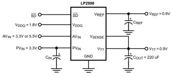
Figure 2. LP2998 DDRII Configuration
