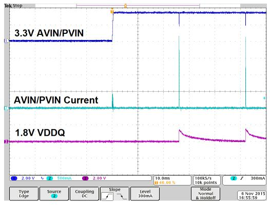
Figure 4. Instrument Cluster DDRII Fault Condition Due to Inrush Current
