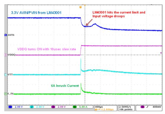
Figure 3. System Shutdown Due to Inrush Current
