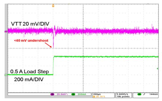
Figure 9. Stabilized VTT with 100m  $\Omega$  ESR in series with 100uF Capacitor
