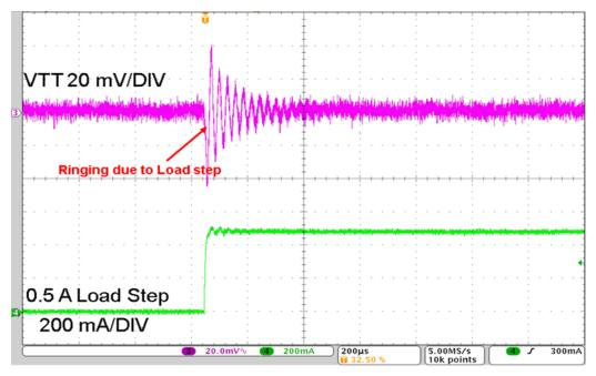
Figure 8. Ringing at VTT of LP2998 with 100uF Ceramic Capacitor
