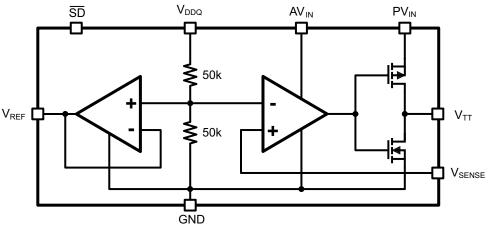
Figure 1. Simplified Functional Block Diagram
